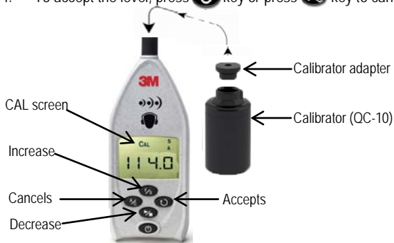
Figure 1-10: Calibrating the SD-200
