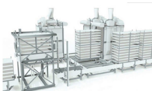
Figure 1: Multistage CO 2 stunning system for poultry
