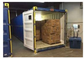
Figure 1: AirWatch GasPod for Shipping Container Measurement
