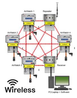
Figure 4: AirWatch mesh network with one receiver, one repeater and four AirWatches.
